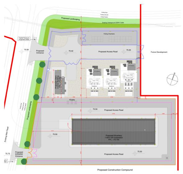
Figure 2 Extract from Drawing no. GIS-KT-Z0-ZZ-DR-A-1003-P4 by Kavanagh Tuite Architects indicating the Proposed Substation Compound, Client Control Building and Transformers Compound
